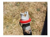
5. Replace the cap on the Dynamic Speed Valve and cover the valves with the flap to prevent water getting inside. Repeat steps 3, 4 and 5 with the other tubes.
